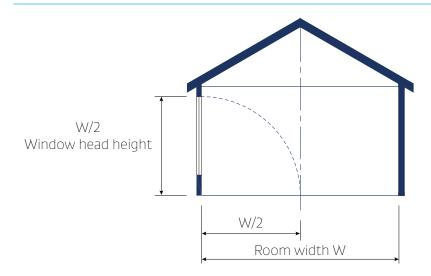
**FIGURE 2.1.2.1B:** Window head heights for windows on opposite side of a room Paragraph 2.1.2.1 c) ii)
