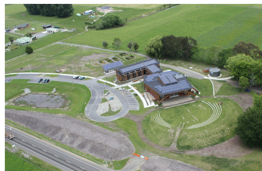
Fig.12. Te Kura Whare utilises a storage pond and landscaping to retain and redirect water.
